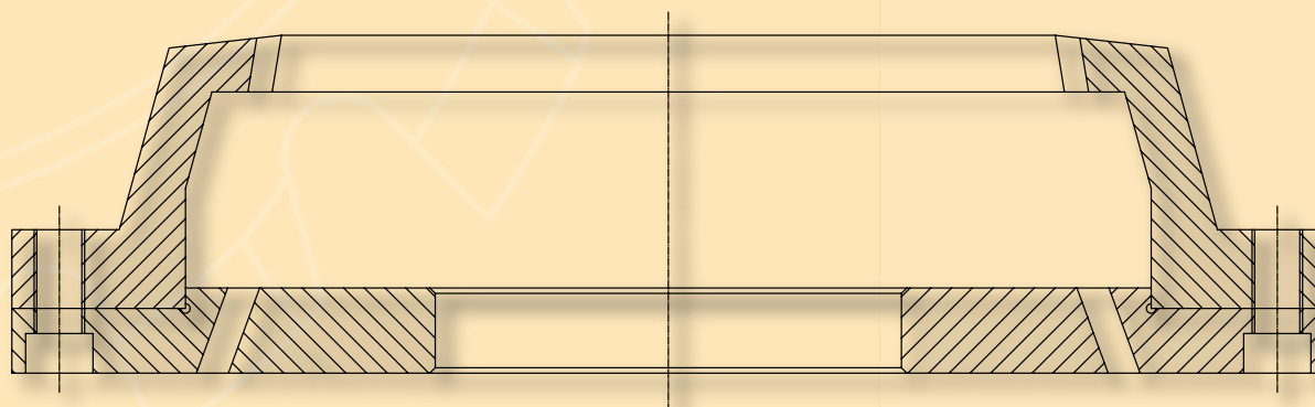
Internal toothed gear shaper cutter for external parts where an interference prevents the use of a conventional disc cutter, and more efficient than a small shank cutter. As with cutters with external teeth these cutters are fully generated to allow resharpening throughout the life of the cutter.
